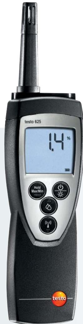
The testo 625 is a compact instrument with an integrated humidity probe head for the measurement of air humidity and temperature. The large two-line display quickly and reliably shows humidity, Wet Bulb temperature or dewpoint, as well as temperature.
