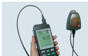
Inspection of transmitters with 4 to 20 mA interface
