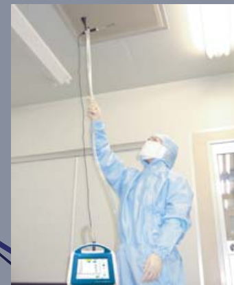
Climomaster™ probe for environmental measurements
